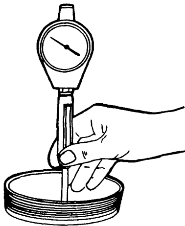
Figure 4-2. Installing Cylinder Meter
